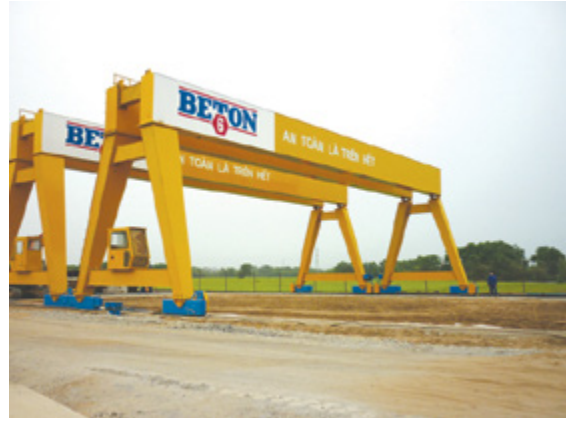
Cổng trục / Gantry Crane Quantity: 34 units Capacity: 3 - 50 tons
