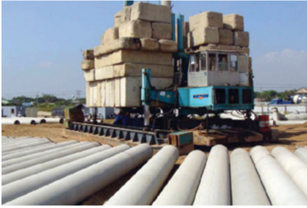
Dàn ép cọc / Pressing Rig Quantity: 06 sets Capacity: 120 - 900 tons
